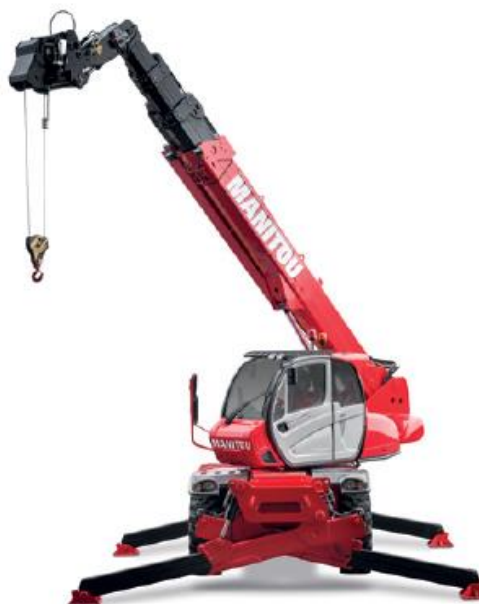
Rotation on lowered stabilizers with 1500 kg jib
